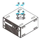
1 Secure the VESA Bracket to the right side panel of the DeskMini 110 series by using the four screws.
