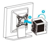
Mount the DeskMini 110 series by turning it counterclockwise.
