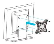
Attach the other VESA Bracket to the rear of a compatible display using the four screws.
